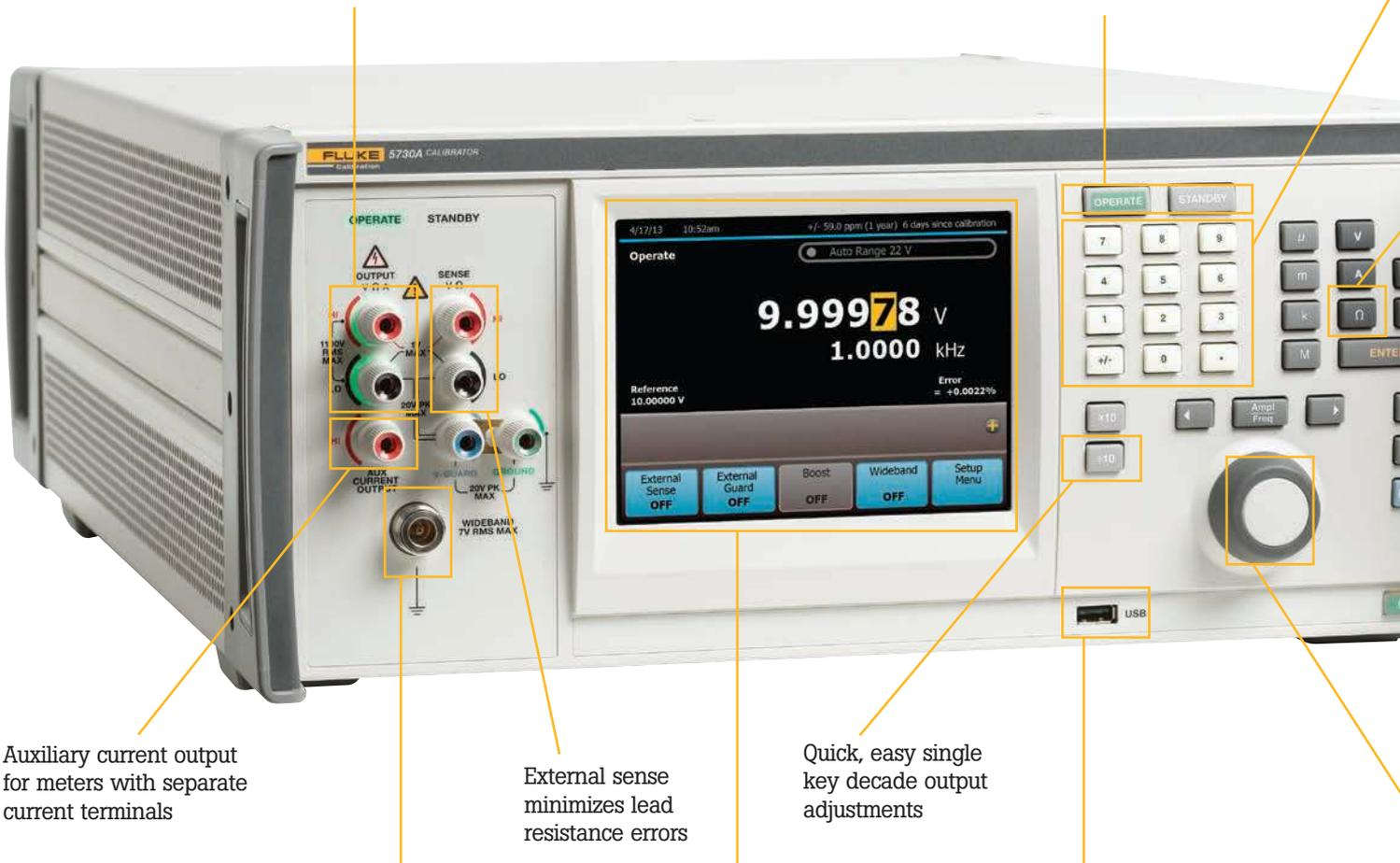
Auxiliary current output for meters with separate current terminals
