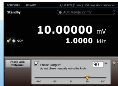
Synchronize and adjust the phase between two calibrators for power meter applications.
