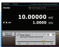
Synchronize and adjust the phase between two calibrators for power meter applications.
