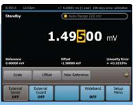
OFFSET and SCALE keys make it easy to compensate for zero offset and scale errors and permit direct display of linearity errors at any scale level.
